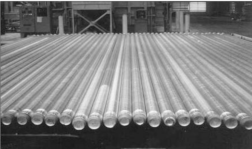
Figure 5.7 Continuously cast semi-solid metalworking feedstock. (Courtesy of Formcast, Inc.)
