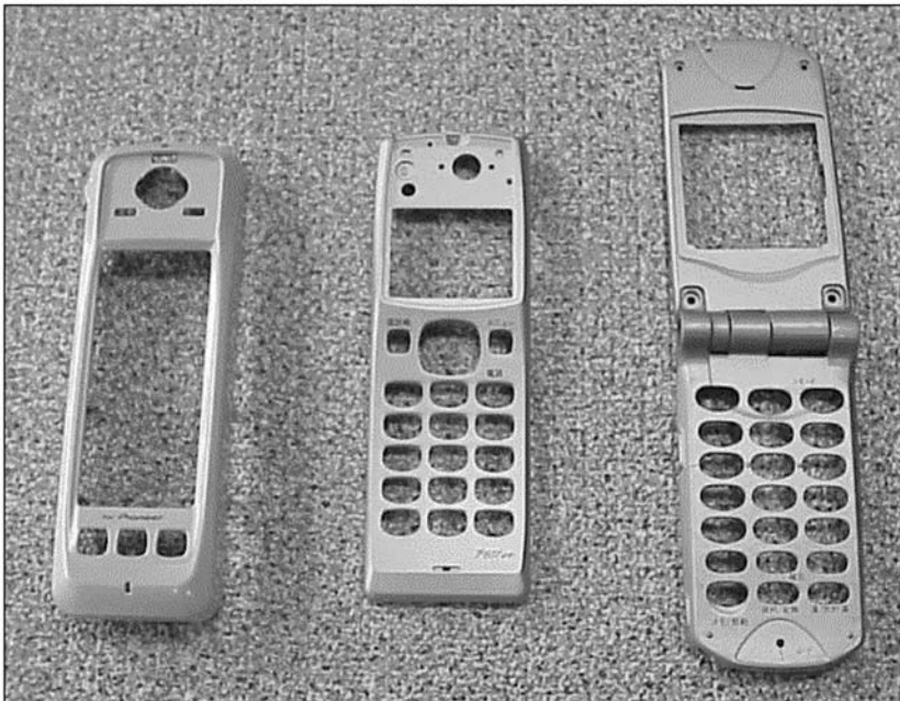
Figure 5.27 Wireless telephone face plates manufactured in magnesium using semi-solid metalworking. (Courtesy of Thixomat.)
