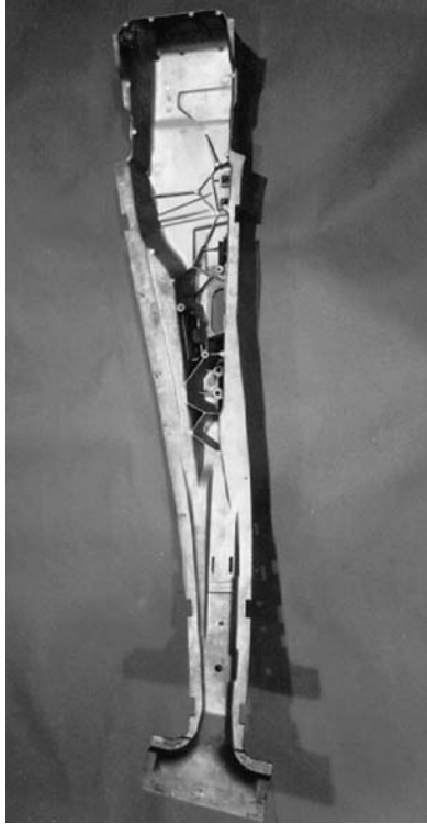
Figure 3.12 Automotive B post manufactured using vacuum die casting. (Courtesy of Formcast, Inc.)
